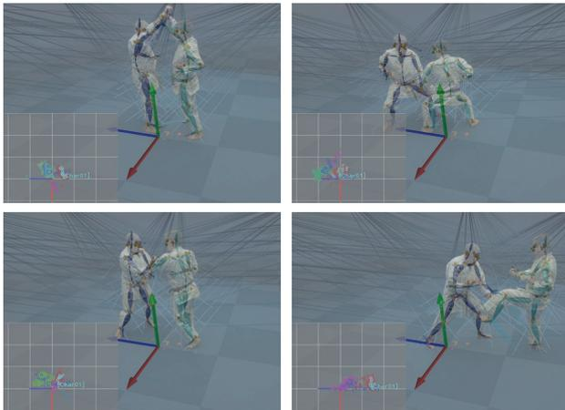
**Fig. 12** Results for four frames of the two-person sequence *Karate*, *Action 13* (8 cameras, 2 × 13 IMUs per subject). Inset are top view visualizations of the subject sorter showing 3D candidates and labelled sorted subjects.
