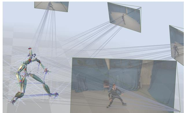
**Fig. 6** Ground truth optical skeleton (yellow) and the solved skeleton (blue) overlaid along with visualizations of the CPM detections from each view back-projected with a line showing where each detection is pulling the corresponding track target. The proposed robust cost function yields a high-quality pose estimate despite several views containing misdetections (*e.g.* swapped feet). Sequence: *Total Capture*, S5, FS1.
