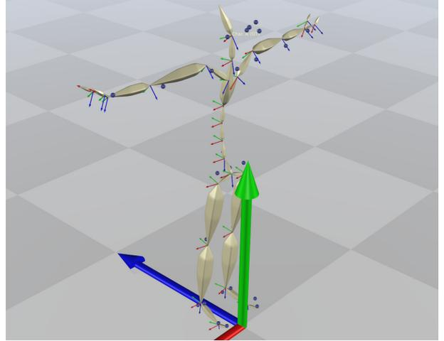
**Fig. 4** Visualization calibrated positional track targets (blue) offsets for the CPM Body25 keypoint set w.r.t. the optical reference skeleton (yellow). Note the offset for both the surface and the joint keypoints.
