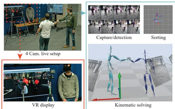
**Fig. 15** Light-weight live implementation of the proposed approach with 4 camera capture and solving running on a single laptop PC (capture area approx.  $3 \times 3$  m). The solved motion is streamed live to a game engine environment on a second laptop and displayed on a virtual reality headset.
