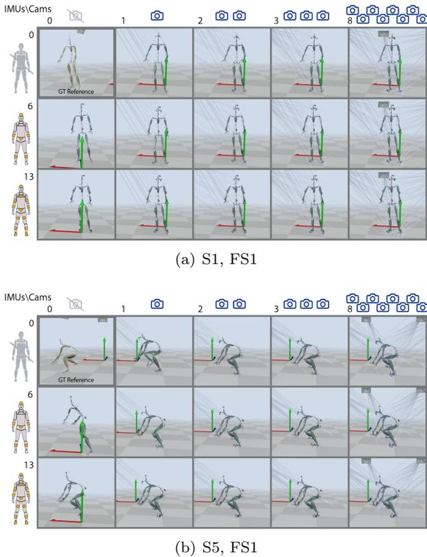
**Fig. 8** Visualization of results of the proposed approach for *Total Capture* S1, FS1 (a) and the more challenging S5, FS1 (b) over a range of input configurations. Note how the quality of the solved pose degrades gracefully as the input is made more sparse.
