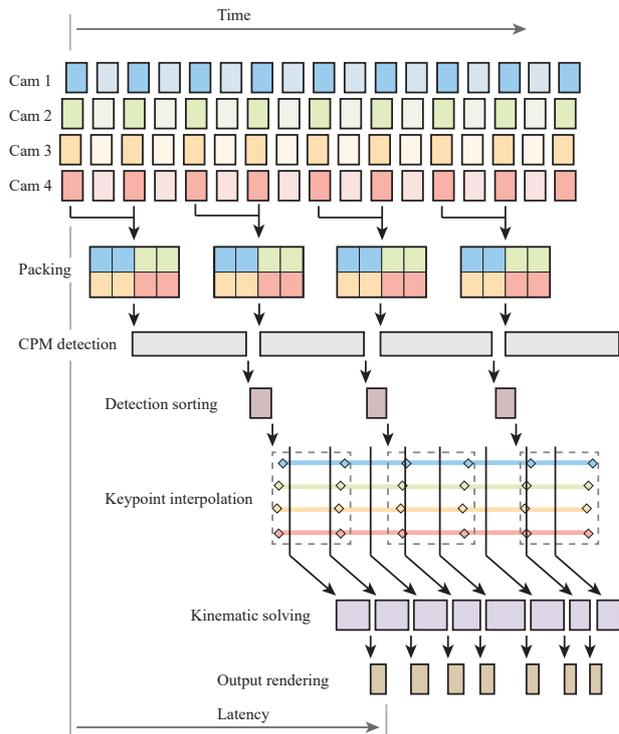
**Fig. 5** Processing flow for live operation showing 4 camera capture, packing multiple frames into single images, CPM detection, detection sorting and interpolation for input into the kinematic solve (timing not shown to scale). Note that the cameras are not assumed to be synchronised, and that the cameras may operate at a higher frame-rate than the CPM processing achieves, as illustrated here by the alternate greyed-out frames in the capture sequence.
