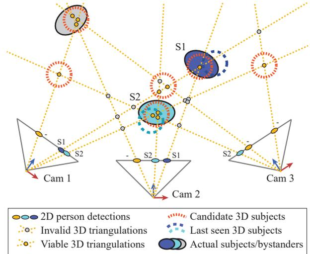
**Fig. 3** Visualization of the proposed approach to sorting and assigning 2D detections to tracked subjects. All possible pairings of detected person instances across views are tested for image re-projection error. Triangulations with high re-projection error are regarded as invalid, while viable triangulations are clustered into candidate 3D subjects. Finally, each tracked subject is assigned to the candidate 3D subject closest to its last seen location.
