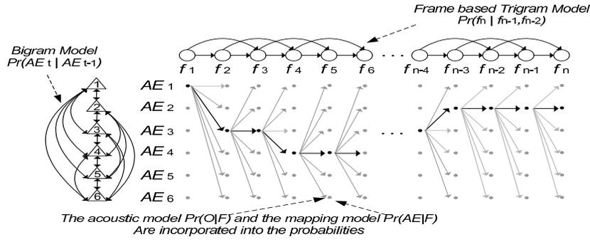
Fig. 1. Viterbi decoding algorithm
