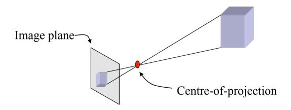
Planar geometric projection - object is projected onto a plane
