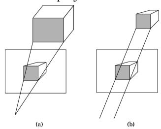
Object distortion can be described by a Homogeneous transformation matrix Therefore, we can implement projective normalisation by concatenating the distortion matrix with the projection
