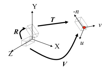
The orientation of the camera is defined by unit vectors n and v which are orthogonal to each other: n.v = 0
