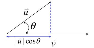
Orthogonal projection of  $\vec{u}$  onto  $\vec{v}$  is:
