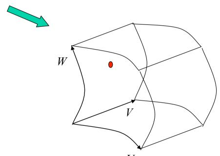
Distorted lattice defined by modified control point positions
