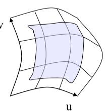
Deformation based on a parametric representation of a surface patch extends directly to parametric representation of a volume
