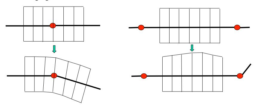
FFD Control Points must be animated non - rigidly to avoid intersection For deformation around a joint
