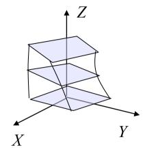
Bend: comprises a bent region + a region which is rigidly transformed For a bend along the y - axis between  $y_{\min} \le y \le y_{\max}$ and the centre of the bend at  $y = y_0$
