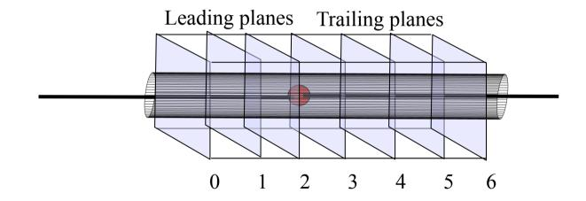
0,1 & 5,6 are adjoining planes - remain rigid to ensure continuity 2,3,4 midplanes - bend to give a smooth surface deformation
